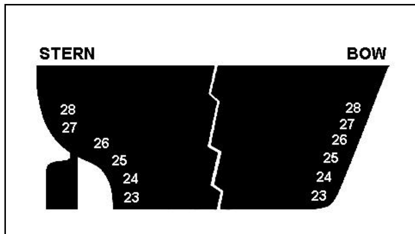
Figure 3-7. Draft Marks on Bow and Stern of Vessel
